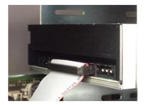
**Power Cable** - Connect an internal computer power supply cable to the power socket at the back of the CD-ROM drive. One side of the plug has chamfered edges, so the power connector fits only one way. Push plug completely into the socket making sure the plug fits correctly.
